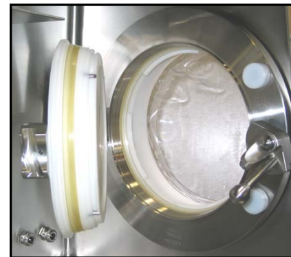
DPTE® transfer system = Double Door Transfer Port (Getinge La Calhène)
