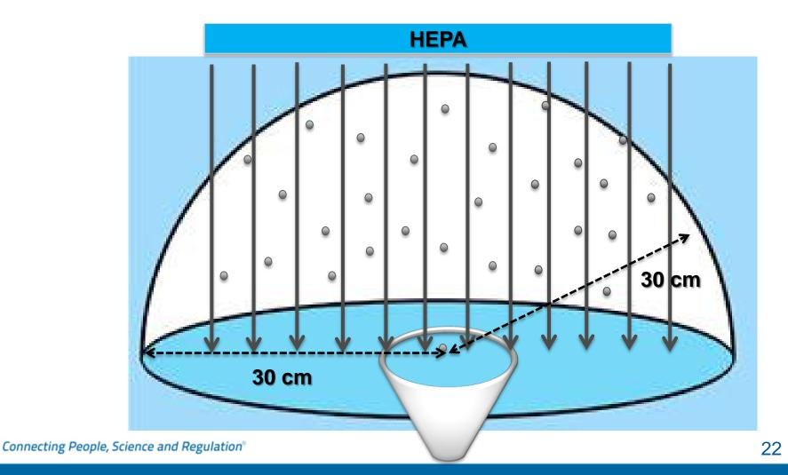
If particles are in laminar air flow, they should follow the pattern and fall vertically, so isoprobe should represend only an air column, not less than 30 cm (1 foot)
