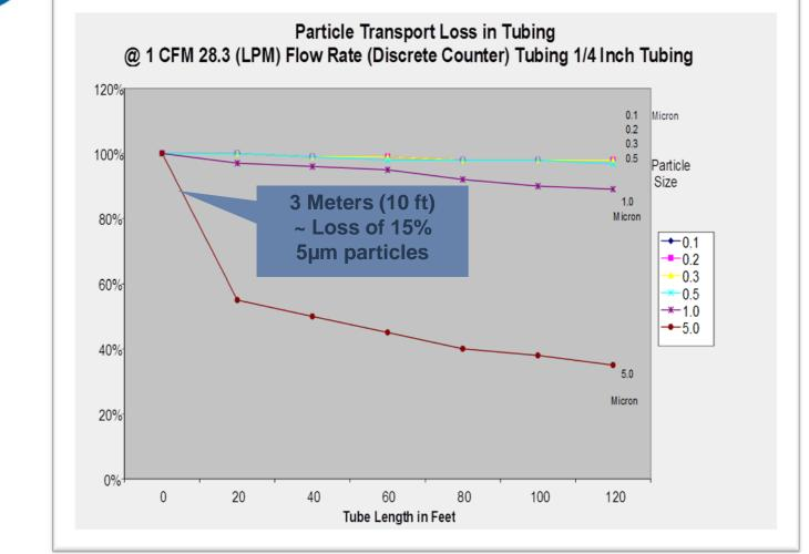
Portable particle counters with less than 3 meters should be used...
